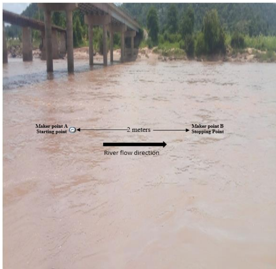
Figure 4. Measurement of water velocity data using Surface Floating Method.
